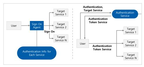
Fig 3. SSO Construction Models
